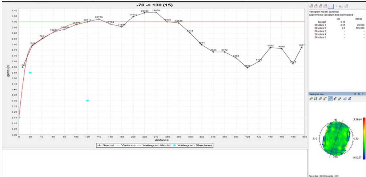
Figure 14.18: Nickel variogram model for the major axis of continuity for the Nose Zone west limb
